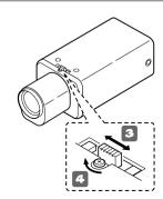
Note: The flange back lock screw is tightened completely when its tip hits the invisible bottom, even though the screw head may seem still up in the air. Do not screw down any further beyond this normal position as illustrated in Fig. 1.
